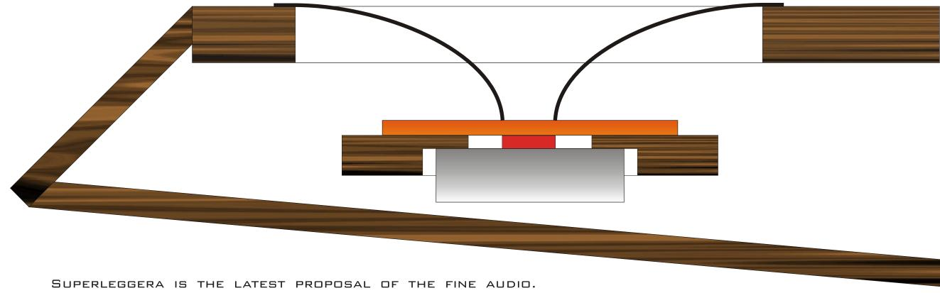
SUPERLEGGERA IS THE LATEST PROPOSAL OF THE FINE AUDIO. THE DRIVER IS BASED ON THE MOVING PARTS OF IMPROVED AUDIO SERIES. THIS NEW DRIVER IS WITHOUT A HEAVY ALUMINIUM BODY. THIS PURPOSEFULLY LIGHT DRIVER HAS NO BODY AT ALL. IT IS SUSPENDED BETWEEN A WOODEN ENCLOSURE AND A NEODYMIUN ENGINE. LIGHTWEIGHT SANDWICH AND WOOD MATERIALS ARE USED TO BUILD A SPEAKER.
